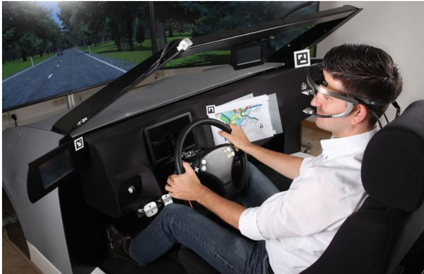
(Eye-Tracking-Marker in einem Fahrsimulatorcockpit)
